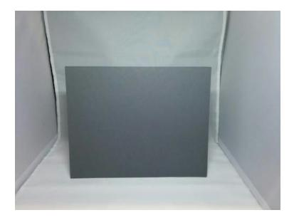
In particular, the grey card is roughly centered in the field of view, taking up around  $\frac{1}{2}$  x  $\frac{1}{2}$  of the scene, with the white background visible on all sides around it. As is evident from the image above, a high degree of precision is not required; the most important factors are that the scene is completely static (including no light source flicker) and that the very center of the image is within the grey card area.
