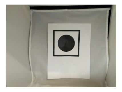
Make sure the square box is completely included in the picture, and no other complicated background is exposed in the scene except the original white one. Place the camera right in front of the test page, so that each of the four edges of the square is roughly parallel to its corresponding border of the picture. Do not point the lighting source directly at the test chart, or allow the black circle to be over-exposed.
