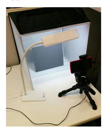
The desk lamp should be reasonably bright: bright enough that it wouldn't be considered a "low light" environment, but not so bright that the device's flash won't make any difference to the scene illumination when turned on. Using the specific desk lamp in this example, setting the brightness to the middle of its three adjustable brightness levels works well.
